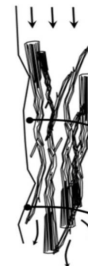
Figure 4. Example conceptual design for headwater channel woody bundle (© Atkins Ltd)
