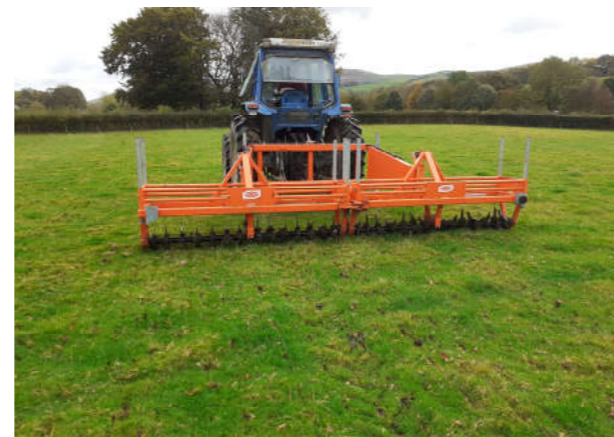
Figure 3. Soil aerator in operation (© Chloe Palmer)
